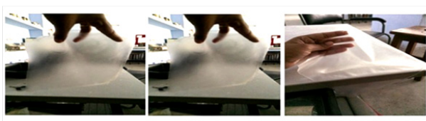
Fig.45. CNF reinforced biofilm from banana starch
